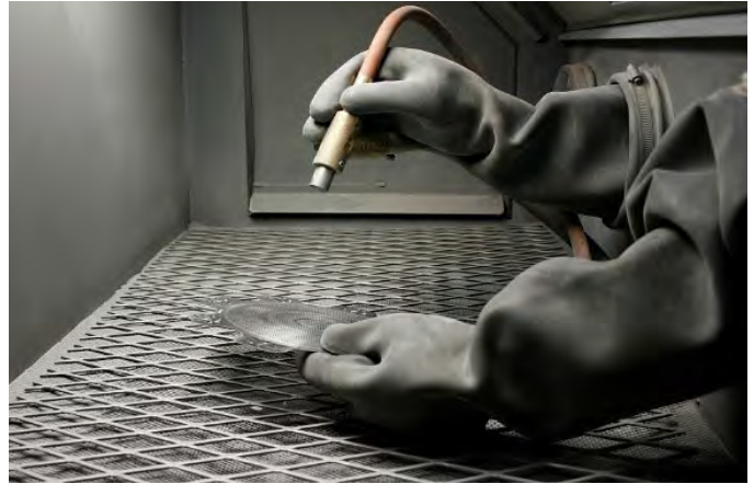
Media blast each side of the grid with consistent motion.
