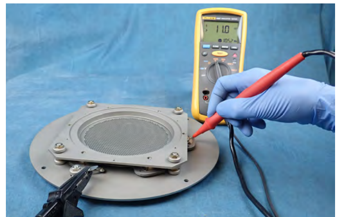
Check isolation on the completed assembly.
