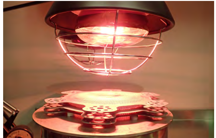
Bake the parts under a heat lamp to remove water vapor.
