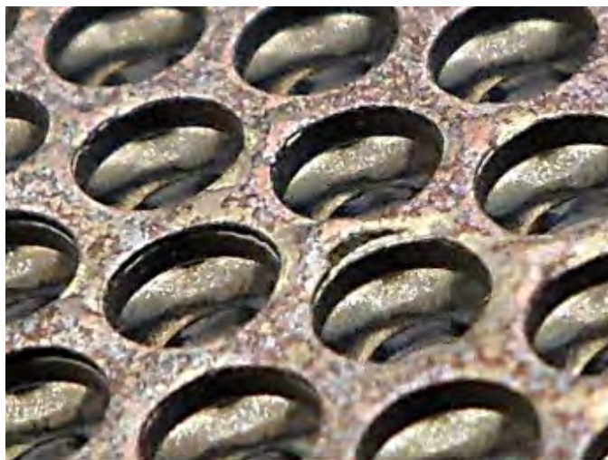
Delamination is where the molybdenum starts to peel back, bubble, and separate between holes.
