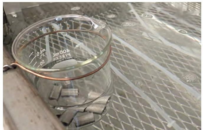
Clean smaller parts in a beaker within the ultrasonic tank.
