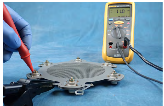
Check isolation on the grid assembly.
