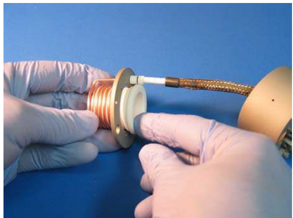
Picture 5.6 – Installing the discharge chamber.
