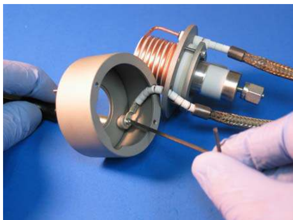
Picture 5.11 – Keeper lead attachment.
