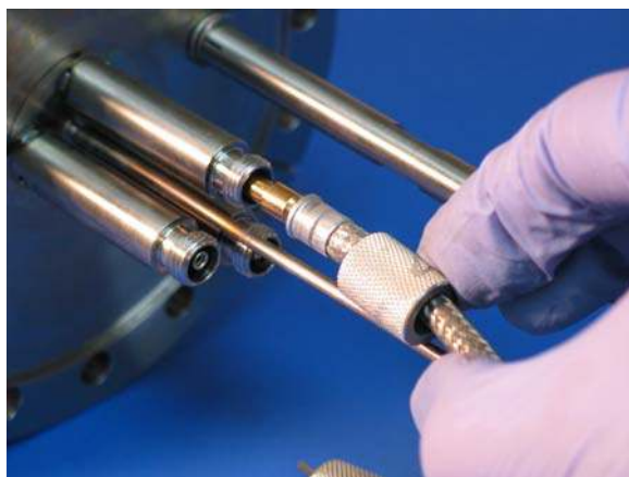
Picture 5.17 – Electrical lead attachment.
