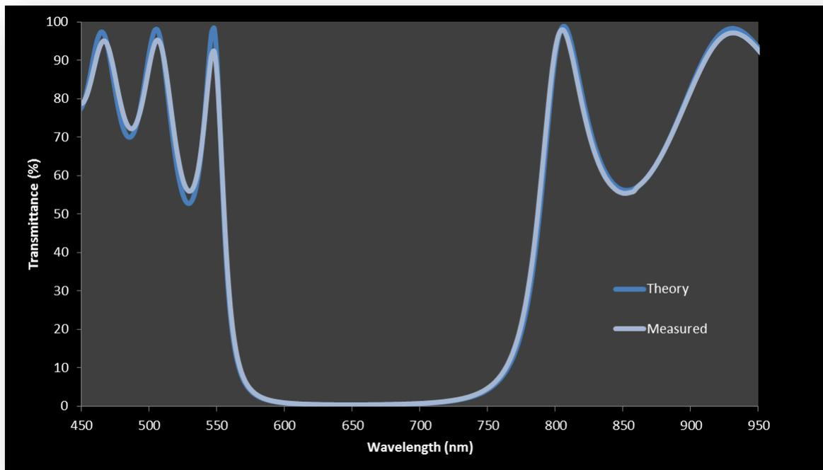
**Figure 3.** Measured transmittance of a typical multilayer mirror filter.
