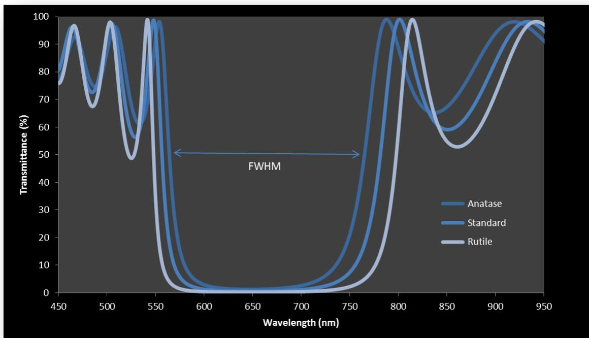
**Figure 2.** Transmittance curves for the multilayer mirror filter
