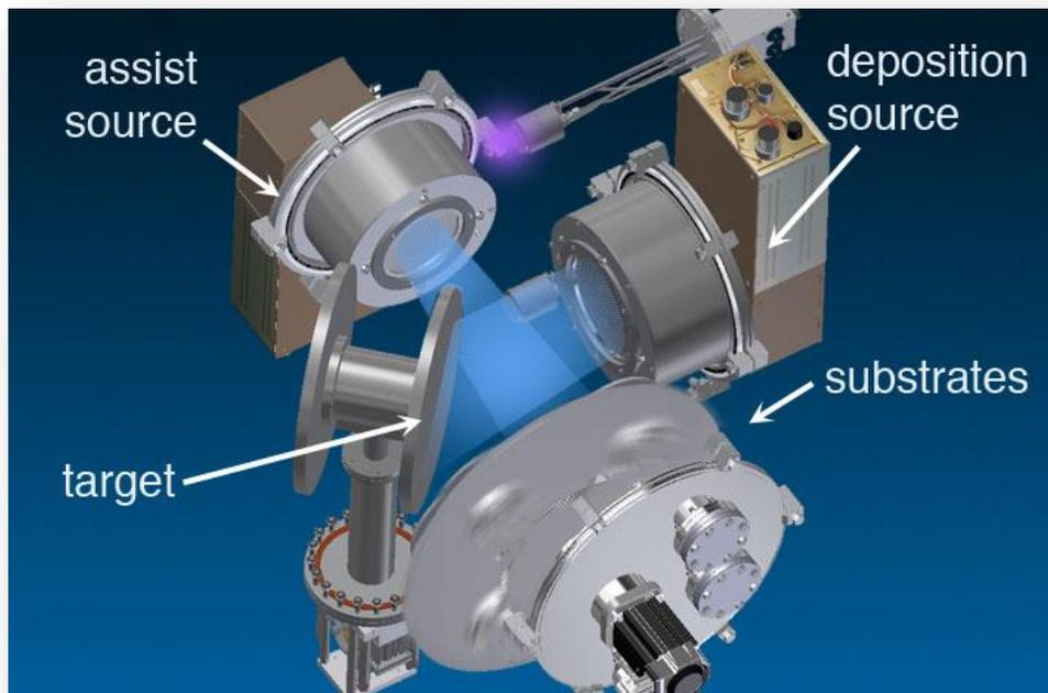
**Figure 1.** Dual ion beam deposition system layout.
