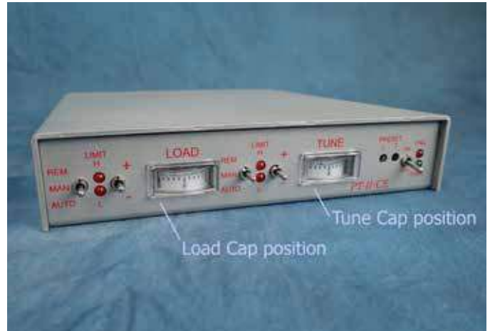
Capacitor position indicators.
