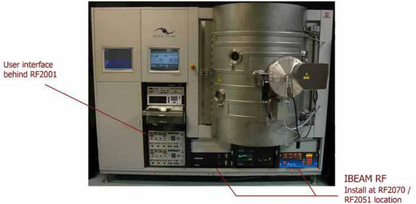
Recommended location for the I-BEAM supply.
