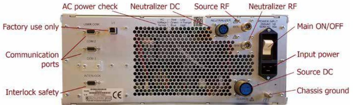
View of the power supply rear panel.
