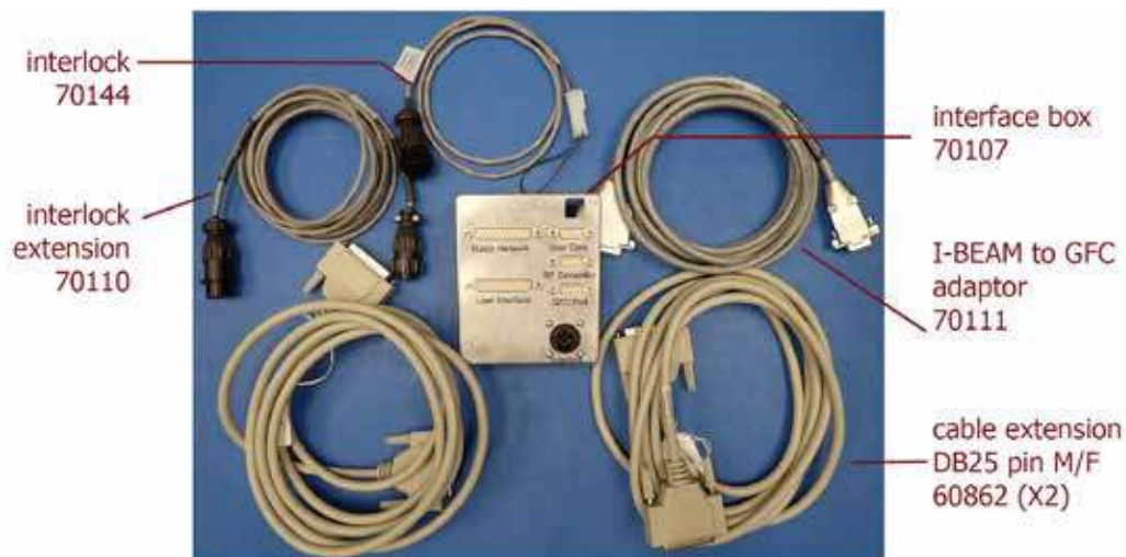
IBOX interface kit for legacy systems.
