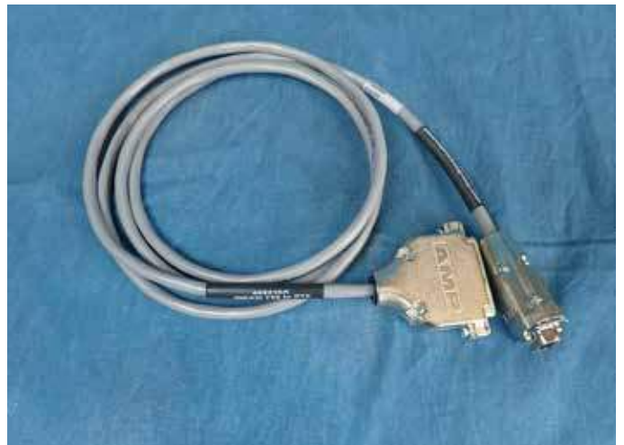
Matching network communication cable.
