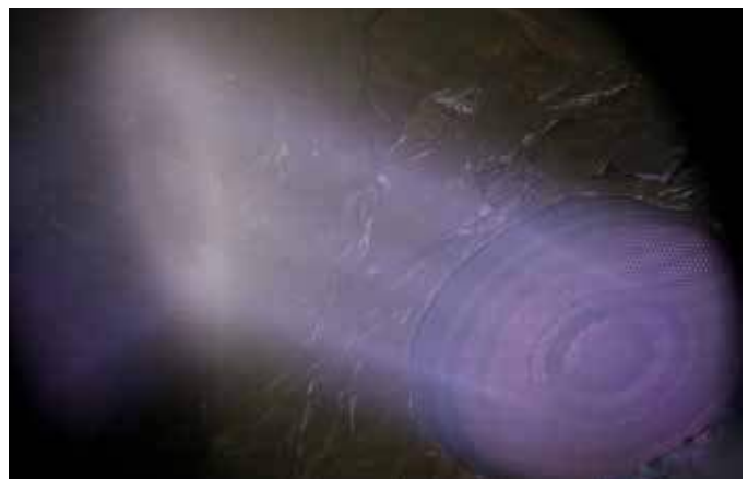
Ion beam striking a target.
