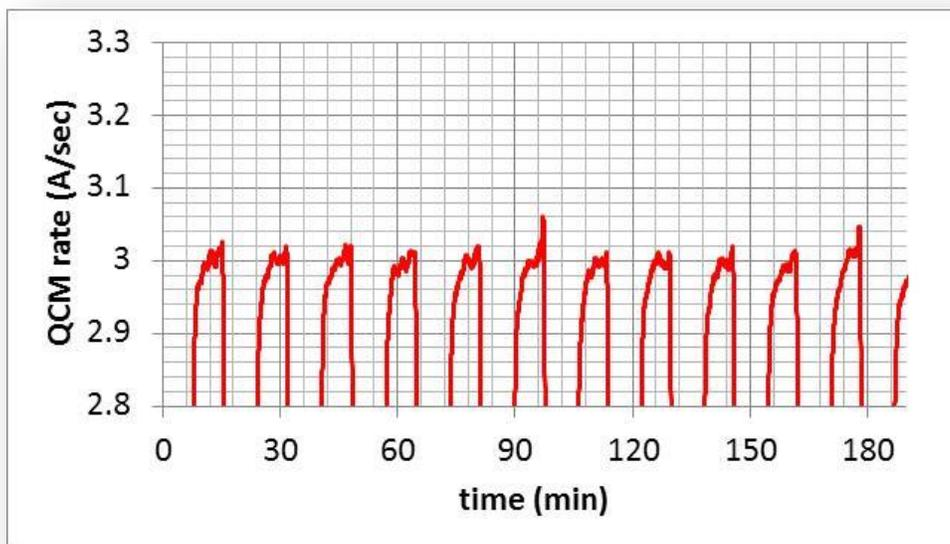
**Figure 3.** SiO<sub>2</sub> deposition rate is stabilized with chamber baking prior to the process run.
