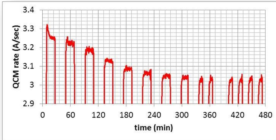
**Figure 1.** SiO<sub>2</sub> deposition rate measured with QCM. Rate decreases by ~7% over the first 300 minutes.
