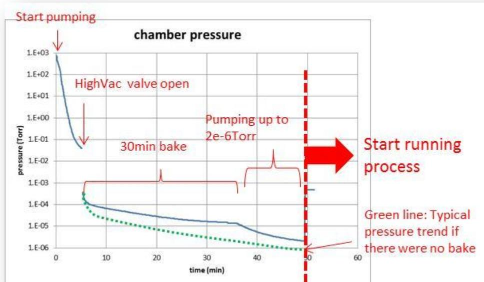
Figure 2. Typical pressure trend during baking step.
