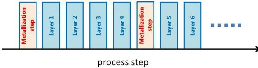
**Figure 3.** An example of the implementation of metallization step. Metallization step is inserted prior to the process run, and every 4 layers.
