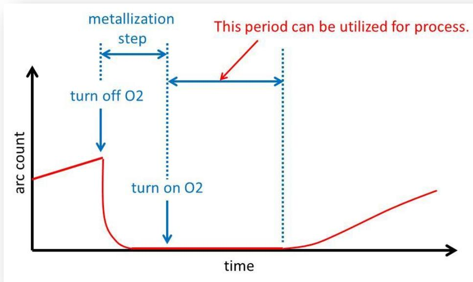
**Figure 2.** Effect of metallization step on arcing. As  $O_2$  is turned off while there is high arc counting, arc count rapidly decreases to zero within a few min. Arc count starts to increase once  $O_2$  is turned on again, but only after some arc-free process time.
