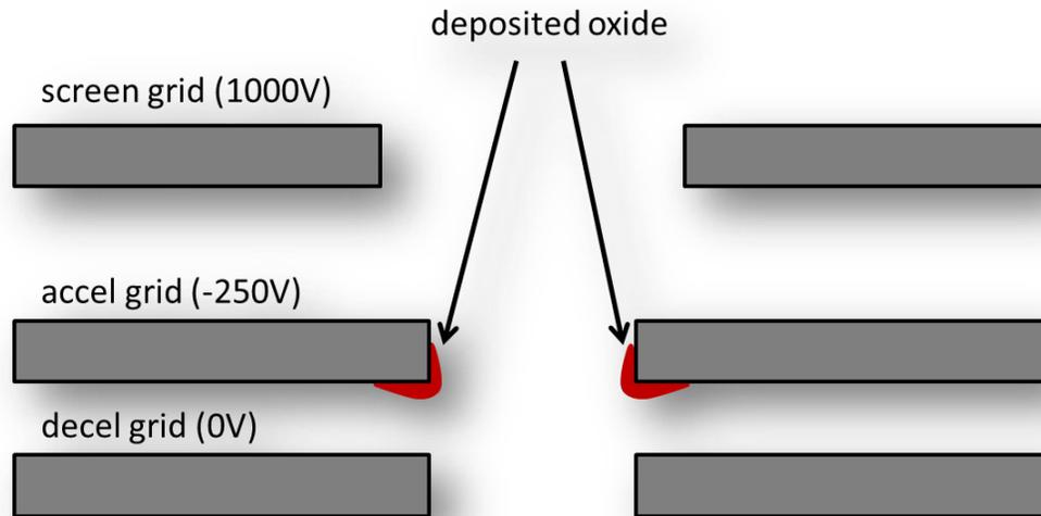
**Figure 1.** Grid assembly beamlet (one hole) diagram with a clean screen and decelerator grids, oxide coated accelerator grid.
