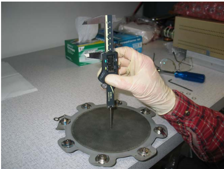
Photo 4: Depth gauge measurement of the tube resting on the screen grid.
