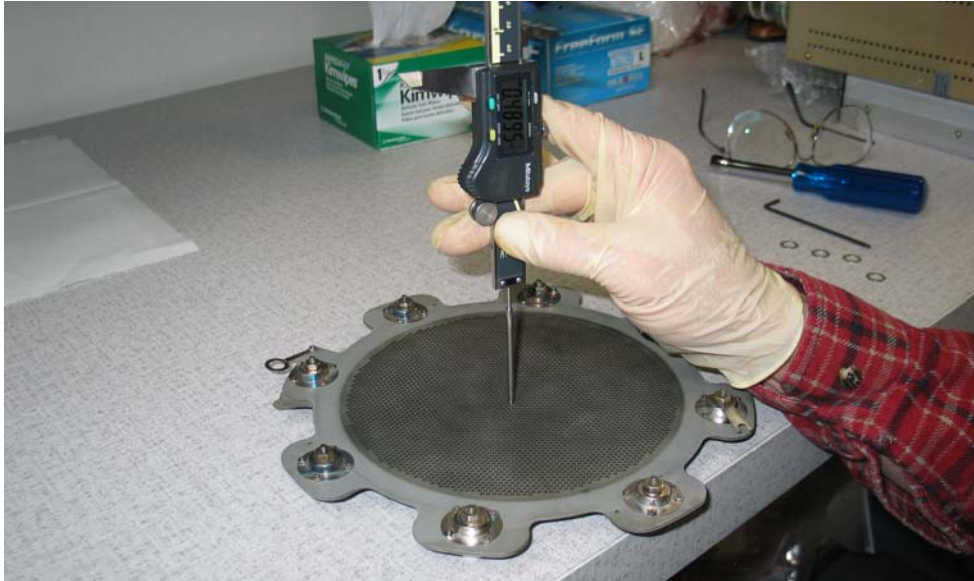
Photo 3: Depth gauge is inserted into the screen grid hole and resting on accel grid.
